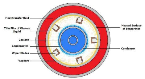
The distance between heated surface of evaporator and cooled surface of the condenser is very short due to which generated vapours of low boiling components gets condensed immediately which minimise the pressure drop and ultimately keeps the purity of condensates high.
